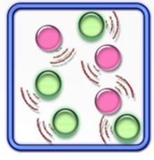
Low Temperature Less Collisions Slow Curing High Temperature More Collisions Faster Curing
