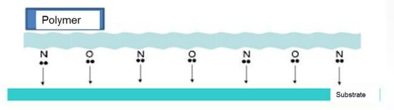
In WB or UV finishes, there is no substrate "attack" (except with acidic monomers as HDODA). In this case the chemical interaction is more dependent on the polymer type, polarity, plasticity (Tg) and flow characteristics as surface tension/substrate wetting, levelling and rheology.
