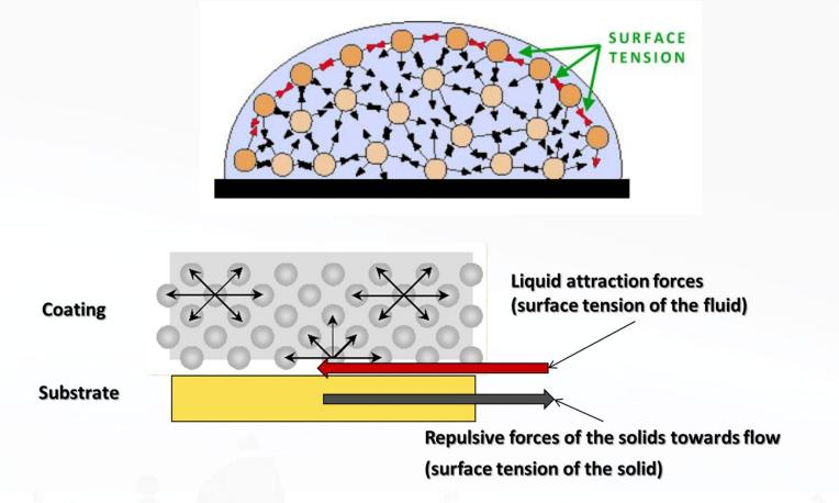
Ideal - Substrate wetting: <u>Substrate Surface Tension > Coating Surface Tension</u> Good film establishment: Adhesion, Leveling, Flow, Gloss, D.O.I. (Image Definition).
