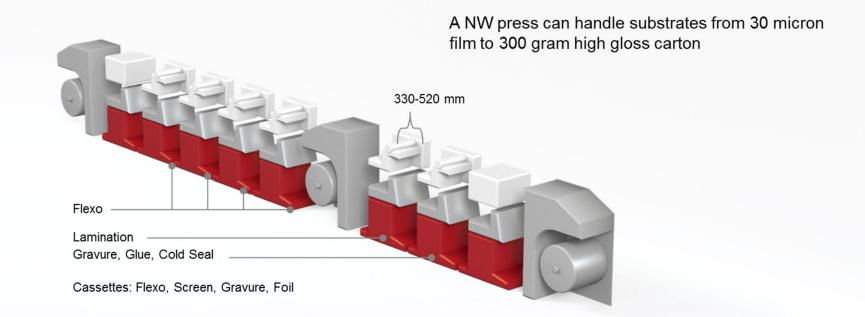
A Narrow web press can contain up to 6 different print methods, and in line finishing like hot foil, embossing, lamination. Converters use the optimal print method for individual jobs. Combining all kinds of print methods, in the same press by using printing cassettes. They may change print method 2-3 times during the day
